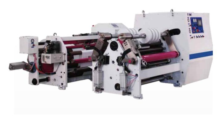
**Main function** Mica tape, insulation material, tipping paper slitting.
